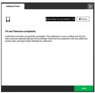
Score of 2-4 indicates that the parts are fitting within the expected tolerances, and you can proceed with normal printing. If score is 1 or 5, please enter score accordingly. Followup to reprint, starting from Step 1.2. (each repeating cycle should move the fiting closer to score 3)
